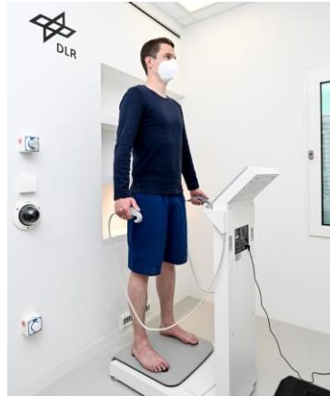
Figure 1: Body composition measurement. Impedance to a small alternating current is measured between electrodes applied at the hands and feet.
